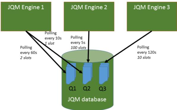
Here, there three queues and three engine nodes inside the JQM cluster. Queue 1 is only polled by engine 1. Queue 3 is only polled by engine 3. But queue 2 is polled both by engine 1 and engine 2 at different frequencies. Engine 2 may have been added because there was too much wait time on queue 2 (indeed, engine 1 only will never run more than one job instance at the same time for queue 2 as it has only one slot. Engine 2 has 100 so with both engines at most 101 instances will run for queue 2).
